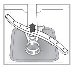
The lower sprayer arm can be removed by pressing on the side tabs and pulling it upwards.
